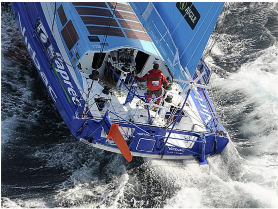
While these arrangements in the open classes with such significant beam may not be so critical, as the static waterline is still likely to be well below the companionway openings, even at ninety degrees knockdown. Below is a picture of a Volvo 60 suffering a knockdown.
